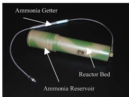
Fig. 1. The ammonia hydride hydrogen generator.
